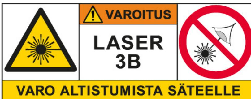
b) Examples of alternative combination signs with the warning sign for laser radiation and a Safety Class 3B warning text. (lasersäteilyä = laser radiation, varo altistumista säteelle = avoid exposure to beam, luokan 3B laserlaite = class 3B laser product, varoitus = warning)
