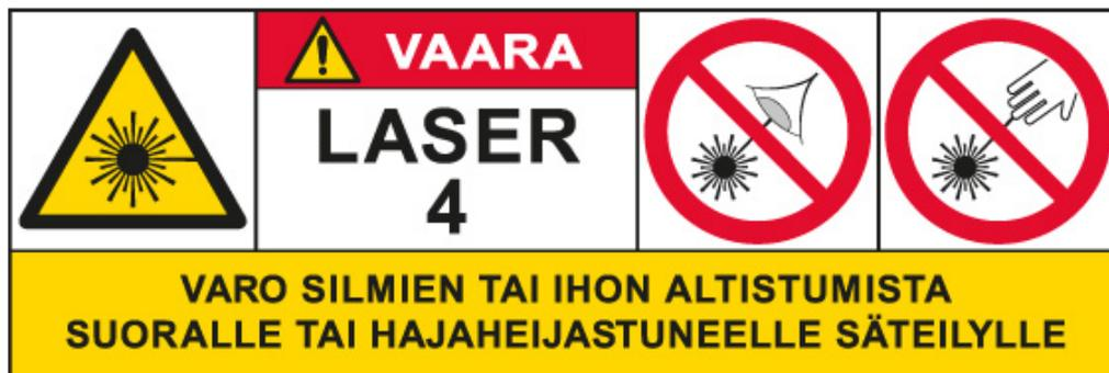
c) Examples of alternative combination signs with the warning sign for laser radiation and a Safety Class 4 warning text. (lasersäteilyä = laser radiation, varo silmien tai ihon altistumista suoralle tai hajaheijastuneelle säteilylle = avoid eye or skin exposure to direct or scattered radiation, luokan 4 laserlaite = class 4 laser product, vaara = danger)
