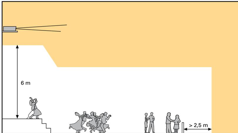
**Figure c).** When unattended beams are used, no laser beams must be present in the area whose safety distances are 6 metres in the vertical direction and 2.5 metres in the horizontal direction (area shown in white in the figure).
