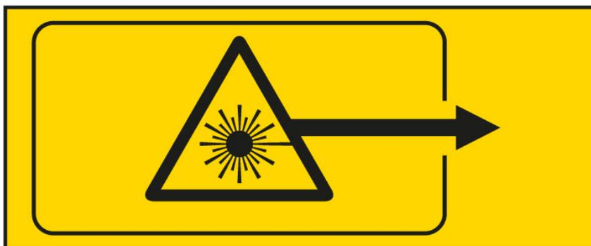
d) Examples of alternative texts or signs indicating the laser aperture.
