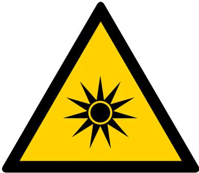
**Figure 9.** Warning sign for optical radiation. If necessary, a supplementary sign must be added to provide information on the type of optical radiation (UV radiation, visible light or infrared radiation).
