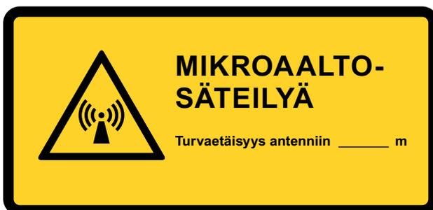
Figure 8. Example of a combination sign containing a warning sign for non-ionising radiation and an explanatory text. (Mikroaaltosäteilyä = Microwave radiation, Turvaetäisyys antenniin = Safe distance to antenna)
