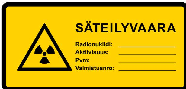
**Figure 4.** Example of a combination sign to be attached to the shield of a radiation source. (Radionuklidi = Radionuclide, Aktiivisuus = Activity, Pvm = Date, Valmistusno = Serial no)
