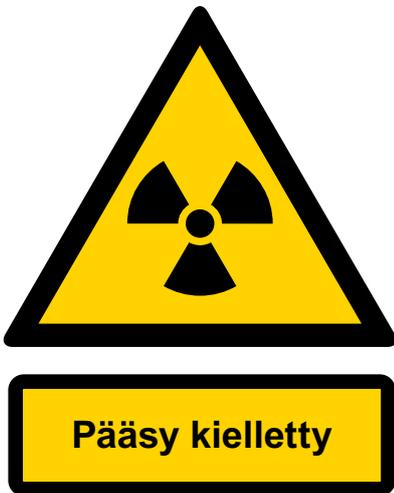
**Figure 2.** Example of a supplementary sign to be used with a warning sign for a radioactive substance or ionising radiation. (Pääsy kielletty = No entrance)
